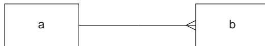
Figure C.20 a is associated with one or more bs . So b has cardinality 1.. with textual form +
