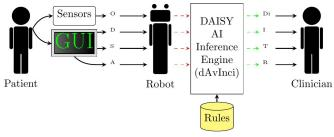
Fig. 3. DAISY workflow: Guided by an autonomous robot, the patient uses a graphical user interface (GUI) running on a tablet computer and a series of sensors to provide Demographic (D), Subjective (S), Objective (O) and Anatomic (A) data inputs, which the robot computer then processes to produce a report comprising Diagnostic (Di), Investigation (I), Treatment (T) and Referral (R) suggestions for an ED clinician to consider.
