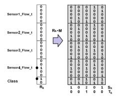
Fig. 2. Diagram showing the use of the CMM for attribute selection. The class attribute is included. The retrieval input vector  $R_k$  is binary for attribute selection whereas Fig. 2 has an integer retrieval vector. The dot is the value for each attribute (a quantisation bin).
