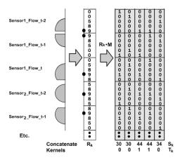
Fig. 1. Diagram showing the application of kernels to a CMM to find the nearest neighbours. The retrieval input vector  $R_k$  is produced by applying kernels. The dot is the bin representing the query value for each attribute. AURA multiplies  $R_k*M$ , using the dot product, sums each column to produce  $S_k$  and thresholds  $S_k$  to produce  $T_k$ .
