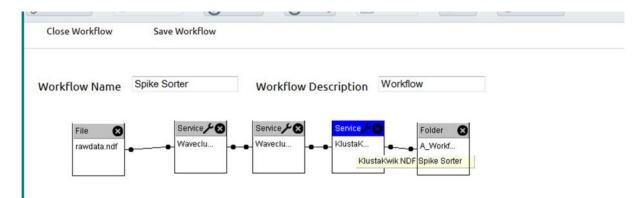
Figure 2 Screenshot of an example workflow for spike detection. The data feeds into a Wave\_clus high pass filter, followed by a Wave\_clus spike detector (Quiroga et al., 2004), the spikes are sorted using a Klustakwik spike sorter (Harris et al., 2000) and the results are output to a selected folder.
