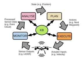
Figure 2: High-level diagram of autonomous drone MAPE-K.
