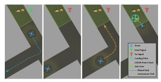
(a) Surveying (b) Signal Loss (c) Return Home (d) Landing Figure 1: An illustration of the return-to-home exemplar problem used to demonstrate our *Aloft* artifact. The drone begins to survey under pilot control (a) but then loses signal (b). It must then autonomously perform a return-to-home function (c) and land safely (d).
