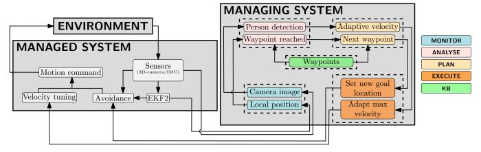
Figure 4: The architecture for the return-to-home behaviour.
