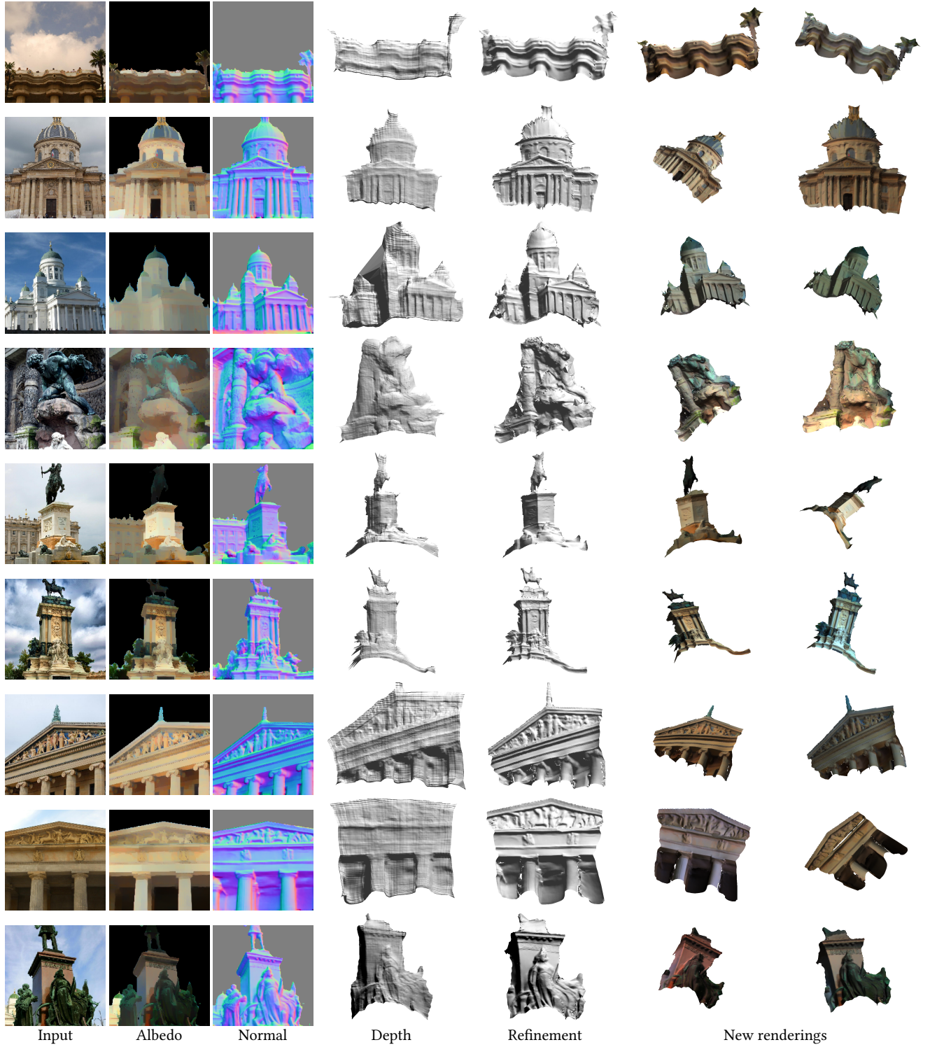
Figure 5: Results of applying our method to images from the MegaDepth dataset [Li and Snavely 2018c]. Col. 1: input image. Col. 2 and 3: albedo and surface normal maps estimated by InverseRenderNet [Yu and Smith 2019]. Col. 4: rendering of the geometry provided by the depth prediction network. Col. 5: refined geometry after merging with the surface normals. Col. 6 and 7: novel views under two different lighting conditions.
